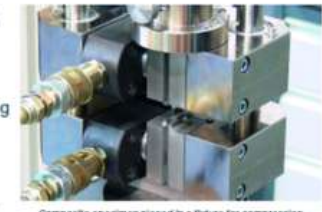
Composite specimen placed in a fixture for compression testing.
