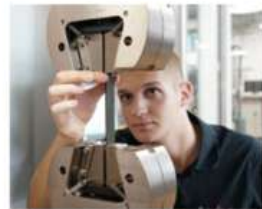
Preparing a composite sample for tensile testing.
