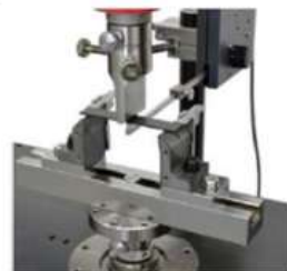
Set up for flexural testing using a 3-point bending fixture.
