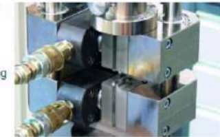
Composite specimen placed in a fixture for compression testing.
