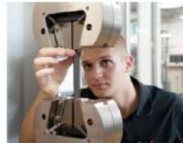
Preparing a composite sample for tensile testing.
