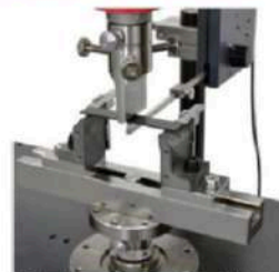
Set up for flexural testing using a 3-point bending fixture.
