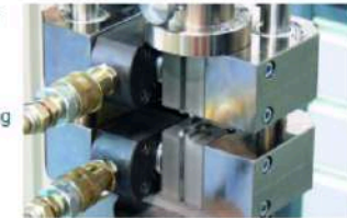
Composite specimen placed in a fixture for compression testing.
