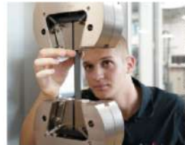
Preparing a composite sample for tensile testing.
